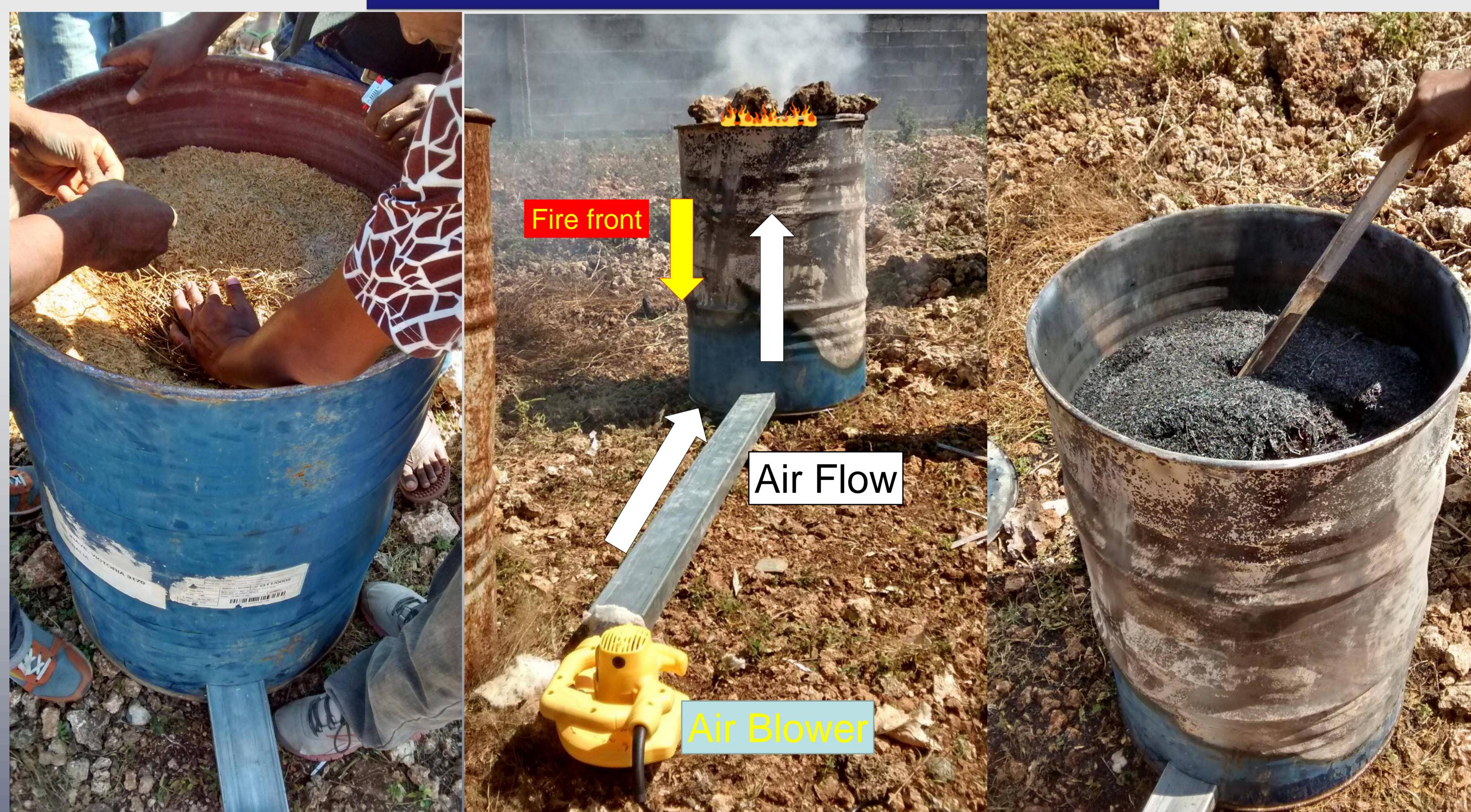
Rice Hulls are placed in drum and lit from the top.
